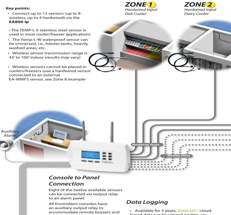
accommodate remote buzzers a strobes (or as an optional single output to the alarm panel).
