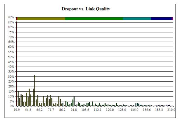
The link quality is a decimal number from 0 - 255; 0 representing low signal quality/strength and 255 representing high signal quality/strength. From the graph, the following observations were made:
