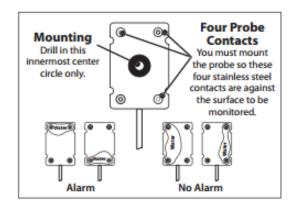
NOTE: The W-UC-S sensor must be connected to an EnviroAlert or WaterBug WB-800 for water detection
